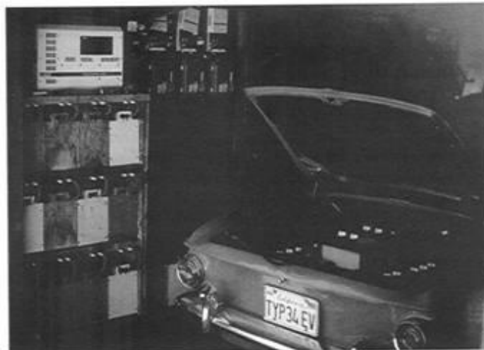
The author's Type III Karmann Ghia charging from a 3 kilowatt photovoltaic array. Batteries and a Trace 4 kW inverter are visible on the wall behind the car.
